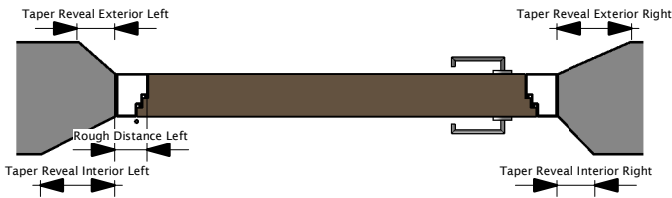
PLAN DIMENSIONS TAPERED REVEALS
